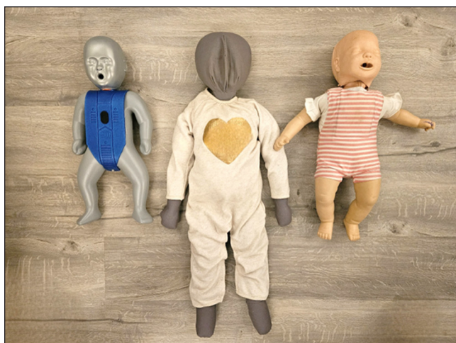
Figure 1: An image of the study manikin (middle), compared to a Vital Signs Inc. ACTAR 911 Infantry (left; later referred to as the “teaching manikin”) and a Laerdal Baby Anne (right).
